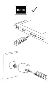
To charge the Plus, remove the mount. Then charge in any USB port.
